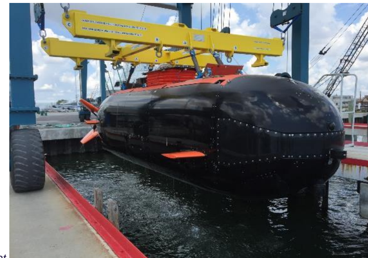
Left: MASTT – Mobile Anti-Submarine Training Target, the world's largest unmanned underwater vehicle
