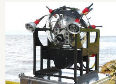
Left: Autonomous robot, designed and deployed for hadal research in the Puerto Rico Trench
